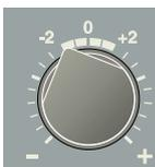
This knob is used to change the heating curve's parallel offset and in doing so the room temperature. Turning clockwise increases the room temperature. When the knob is turned menu 2.0 is shown on the display screen and the value for the calculated supply temperature changes.
