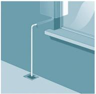
A condensate pipe carries condensation from your boiler to your outside drain. It's usually a white or grey plastic pipe that travels from your boiler through the external wall directly outside where your boiler is located.
